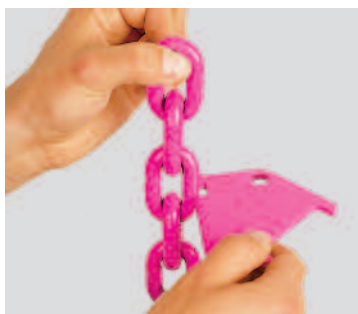
Testing wear of nominal diameter
