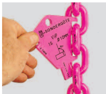
Testing for plastic elongation caused by overload
